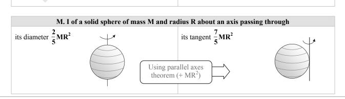
Using parallel axes
